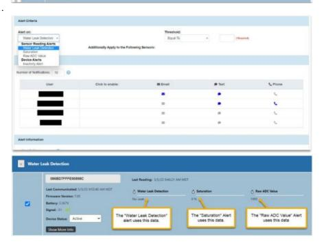
Water Leak Detection Alert: If you want to send an alert when the "Water Leak Detection" is reporting "Leak" set: "Threshold" to "Equal To" and enter: 1 in the next required field.
