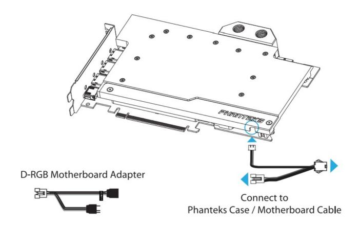
You can connect the D-RGB cable to a compatible motherboard with the D-RGB Motherboard Adapter.
