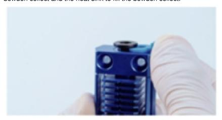
3. Assemble the plunger into the larger hole at the bottom of the heat sink, and screw the flat head screw M3.0'4.0 into the threaded hole on the heat sink with the H 1.5 hexagonal bar (no need to locking), so that the plunger won't fall off. Please note that the hole on the plunger should be directly opposite to the threaded hole on the front of the heat sink, which would ensure that the screw can be smoothly screwed in.
