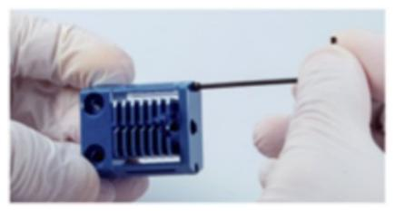
2. Embed the bowden collect into the top of the assembled heat sink, then insert the collect clip in between the bowden collect and the heat sink to fix the bowden collect.
