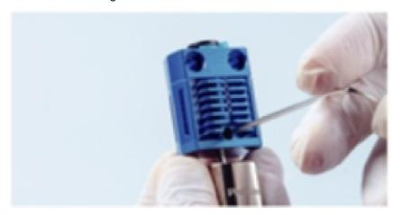
7. On the A side of the heat block. screw 3 flat head screws M3.0'3.0 into the 3 threaded holes respectively with the H1.5 hexagonal bar.
