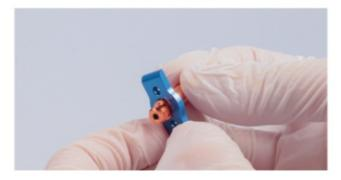
3. Screw the heat break into the side – A of heat block by using 5mm open – ended wrench (Attention: Side – A of heat block should be completely attached to the heat break).
