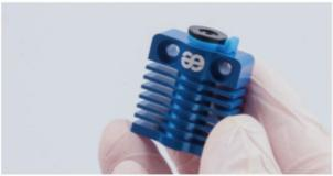
2. Assemble the heat sink rib through the threaded end at the bottom of the heat break, to the middle of the heat break (Make sure the side of the countersunk hole of the rib is toward the threaded end).
