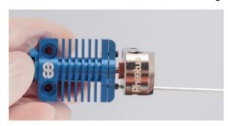
6. Screw two M3 head screws into the correct holes on the B – side of the heat block respectively by using 1.5 hexagonal bar.
