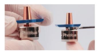
4. Put the heat break and heat block into the heat sink (Attention: Ensure that the holes on the rib are aligned with
