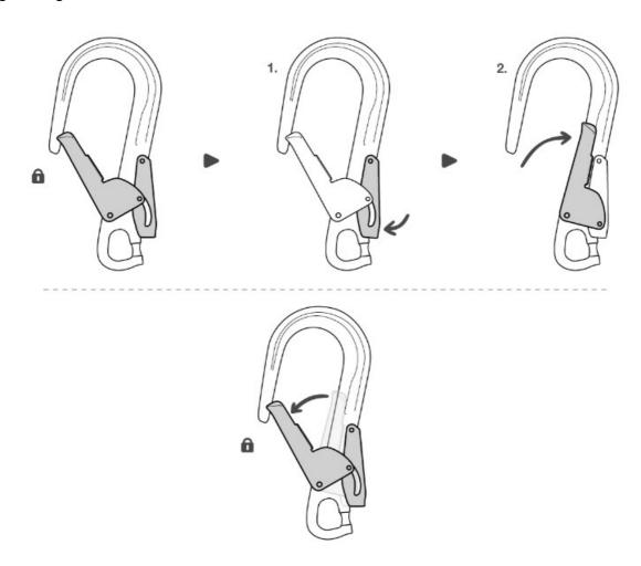
Personal protective equipment (PPE) used for fall protection from height. EN 362: 2004 connector – classes A/T (anchor/manufactured termination). Auto-locking carabiner designed for activities with a risk of falls from height. This product must not be pushed beyond its limits, nor be used for any purpose other than that for which it is designed.
