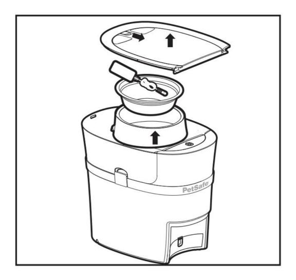
2. We recommend you wash and rinse the bowl, bowl holder, food hopper, lid and conveyor. Once parts are dry, ensure a conveyor belt lip is aligned with the arrows on the side. Replace the conveyor and food hopper.
