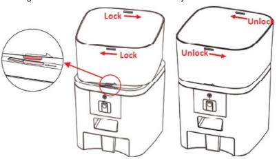
Put the desiccant pack into the drying box on the top cover. Unlock the lock on the cover to install the cover. Then place the feeding tray into the feeder from the bottom. Rotate the lens down to monitor feeding tray.
