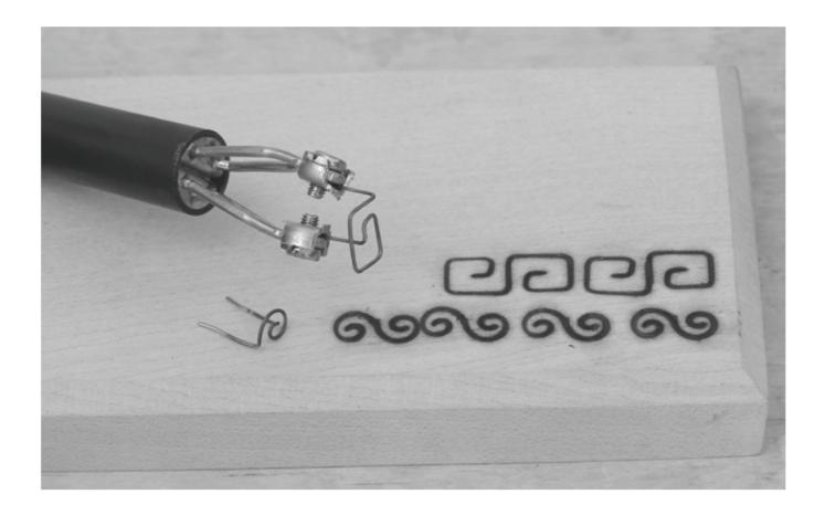
Small brands can be shaped from wire and used for repeat decoration. These are formed by using small pointed pliers and must be accurately made so that the whole of the pattern touches evenly in use. 23 S.W.G. wire is needed for rigidity.
