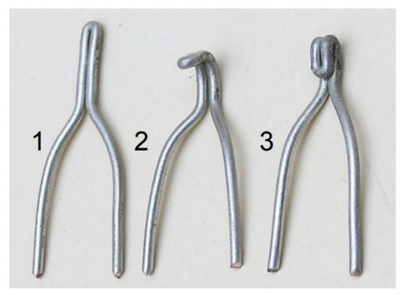
whilst red hot, using pliers. It might be thought that the current would be shorted out where the loops touch and this may well happen with a newly made point, but in a short time a coating of oxide will form which insulates the wire and then the point will brighten up visibly.
