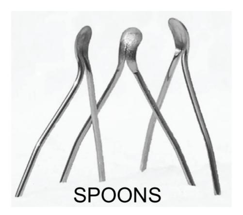
A large area of contact with the wood is required for efficient shading. A spoon point (shaped like a miniature SPOONS a standard point can be hammered price list) can be used or a standard point can be hammered out flat on a hard metal anvil such as the head of a hammer held in a vice. If necessary any sharp edges can be removed by rubbing on abrasive paper.
