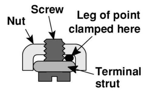
The wire must be clamped between the terminal strut and the nut, not under the screw head. Tighten the terminal screws taking great care not to bend the terminal support struts. Squeeze the point into shape with pliers if needed. You can buy a spare pencil to hold a different point and plug it into the transformer when needed rather than having to continually change points on the pencil.
