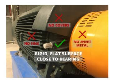
Use the rotary tool to strip the paint from the mounting location on the machine.
