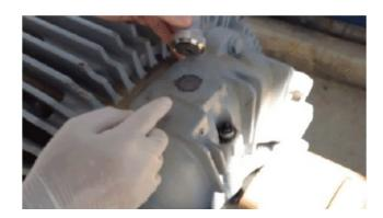
**Note:** The Mote must be mounted with the Petasense logo facing the direction of the machine's shaft for orientation purposes
