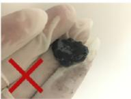
Roll epoxy into a 2-3 inch strip, then form a ring on the bottom of the Mote mount.
