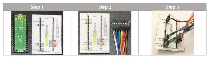
4. Connect the other side of the bridging cable to the EXT3 board (Step 4 and 5). There is a black mark on the EXT3 for pin 1 and a white one for pin 10.
