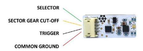
The Plug that is used in G&G replicas with ETU and works with Perun ETU++ is JST ZHR-4. It is available in many electronic shops. We recommend using plugs with pre-installed wires that can be lengthened, because correct preparation of the bare plug might be difficult. The correct plug wiring order is shown here.
