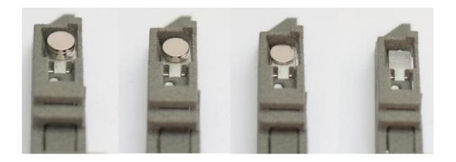
Note, that using these magnets with steel AK receivers will cause Clicker to become locked! However, this can be worked around by gluing a piece of non-ferromagnetic material to the top magnet, so that it does not stick to the receiver. Keep in mind, that with such solution the overtravel will be additionally limited.
