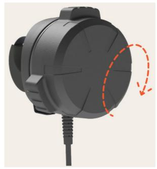
2. Press against face of SpeedControl until LED turns on.
