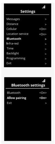
From the Bluetooth settings menu, you can turn on or off Bluetooth mode and Allow pairing. To pair a Bluetooth device with your wheelchair, follow the instructions for Bluetooth pairing setup and pairing with a device. See 2.8.2 Pairing setup and 2.8.3 Pairing with a device.
