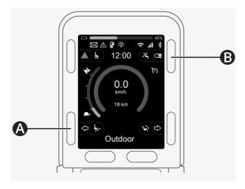
If more than one paired Bluetooth device has its Bluetooth enabled, the screen shows a list of paired devices. To connect and use a paired device, select the device's ID and deflect the joystick to the right.
