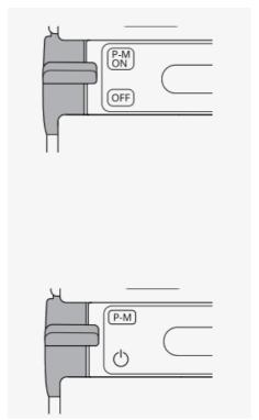
The paddle switch can also be used to scroll through the available profiles and modes. Push the paddle forward to scroll through the available profiles and modes.
