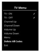
To delete all infrared codes stored in the control panel, select Delete All Codes in the infrared setup menu.
