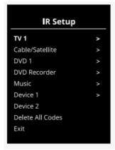
When a command is followed by a check mark it means that it has a stored infrared code. When a command does not have a check mark, its infrared code has not yet been stored.
