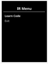
Point the TV remote control towards the control panel's infrared receiver and press the channel up button twice. If the learn code operation has been successfully completed, a green check mark will be displayed on the screen.
