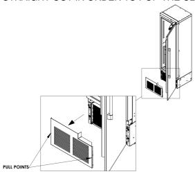
**STEP #2:** SELECT THE CABINET THAT WILL BE PLACED ON THE RIGHT SIDE. SECURE (1) 1013719-1 TO THE FRONT BASE WITH (2) 1008781 SCREWS.
