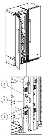
STEP #7: SECURE BOTH CABINETS TOGETHER AT THE TOP WITH (2) 1013719-1 AND (8) M50050-466 STEP #8: SECURE BOTH CABINETS TOGETHER AT THE BACK WITH (1) 1013719-1 AND (4) 1008781 STEP #9: ONCE ALL BRACKETS HAVE BEEN SECURED IN PLACE, ATTACH THE FRONT GRILLS BACK ONTO THE UNT.
