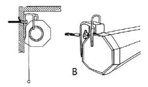
Make sure the screen housing is level to ensure screen material will roll out smoothly.
