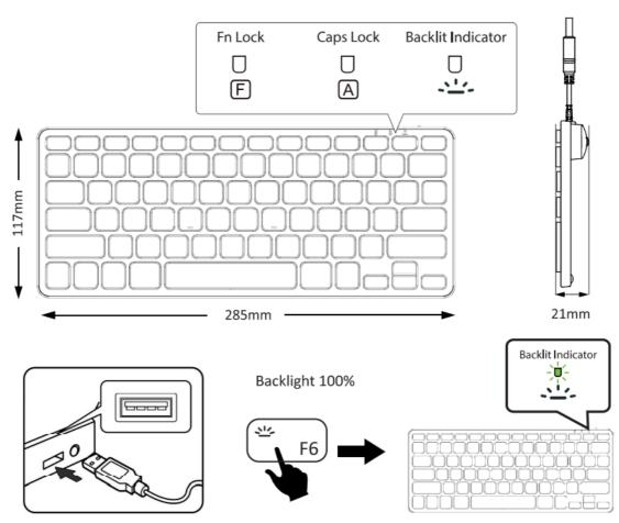
The backlight indicator turns on only when the backlight brightness is 100%.
