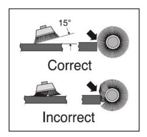
Wire brushes are useful for cleaning and polishing metal, while bristle brushes are suitable for cleaning softer surfaces. As with all rotary tool accessories, you should let the speed do the work without applying excessive force. Use the bristle tips only without mashing the brush against the work piece as shown in the top part of the illustration on the right.
