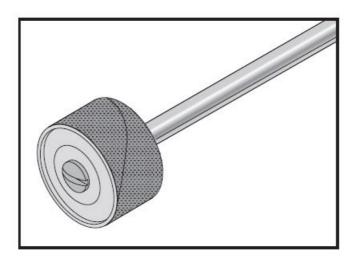
Threaded-tip shanks are used for felt polishing wheels. Shanks with a long threaded tip are used for pointed polishing wheels while shanks with short threaded tips are used for round felt polishing wheels. To install a felt polishing wheel, simply screw it onto the threaded shank.
