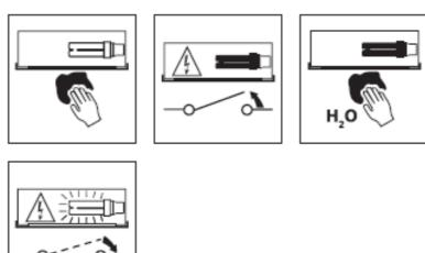
Regularly clean the glass/diffuser diffusor of the spotlight with a soft cloth. – Do not use chemicals for cleaning
