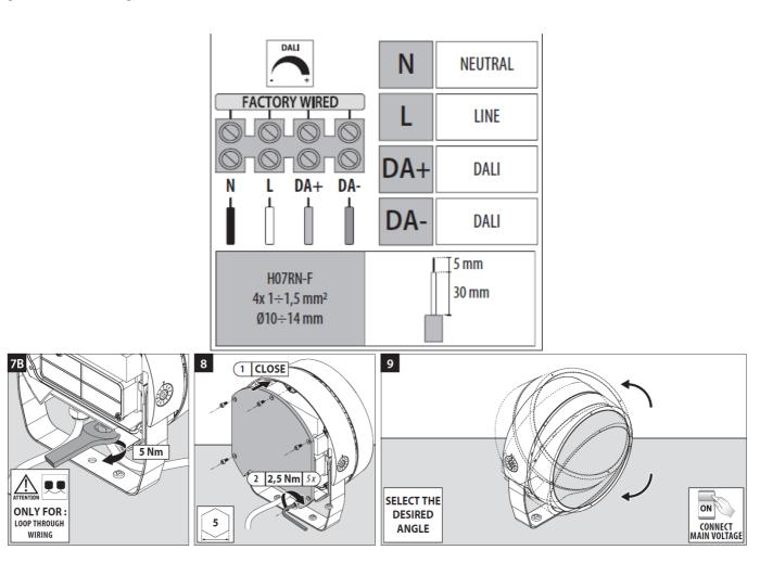
**INSTALLATION INSTRUCTIONS:** The luminaire is suitable for outdoor and indoor installation. – The luminaire is suitable for installation on usually flammable surfaces. – Always verify that the structure is suitable to fix the luminaire.
