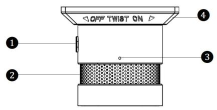
Test Button – Indicator Smoke detector Reset button Mounting bracket
