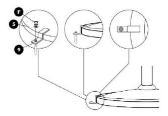
Secure the appliance to the installation surface.
