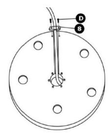
While holding the appliance, fix the power cord to the base.
