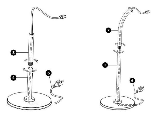
Screw the middle pole onto the bottom pole. Lead the power cord through the middle and bottom poles. Screw the top pole onto the bottom pole. Lead the power cord through the top pole.
