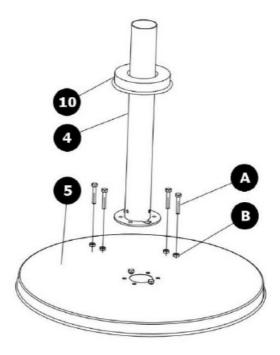
Fix the bottom pole onto the base using the appropriate screws and bolts. Next, slide the cover ring onto the base.
