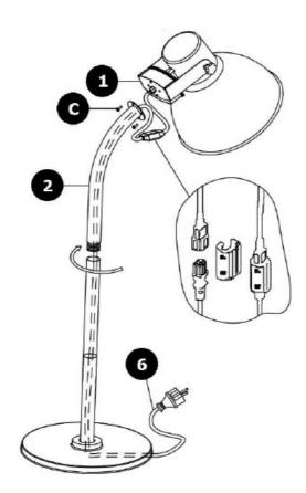
Interconnect the power cord and lock into the box. Fix the head to the assembled poles.
