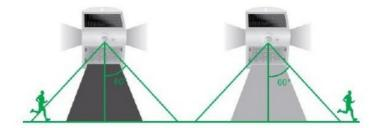
2. Press the mode button twice to enter mode B. This mode automatically switches on to full brightness when a motion has been detected. It switches off 10 seconds after the last motion detection.
