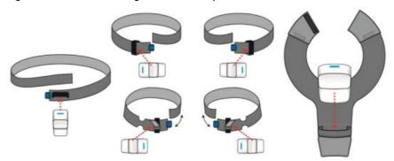
9. Once sensors are placed in the bands, put each band onto its corresponding body part (see image below).
