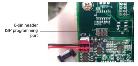
4. Connect the 6-pin ribbon cable connector to the ISP (on the System Programming) port with the RED stripe toward the left-side as shown below.
