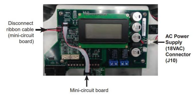
3. Locate the 6-pin header labeled ISP in the upper-left corner of the IntelliChem Controller circuit board (as show below).
