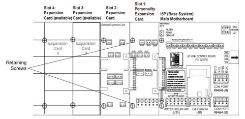
6. When finished, close the hinged control panel and secure it with the two retaining screws. Reinstall the High Voltage Panel and insert the panel's three tabs into the lower slots on the enclosure. Secure the panel with the two (2) retaining screws. Close the front door and secure with the latch. See page 2 for illustration).
