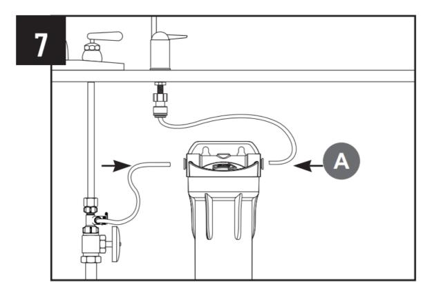
A. Assemble tubing with system as shown in Figure 7, inserting supply adapter tubing into inlet and faucet tubing into outlet quick-connect fitting approximately 5/8-inch until it stops.
