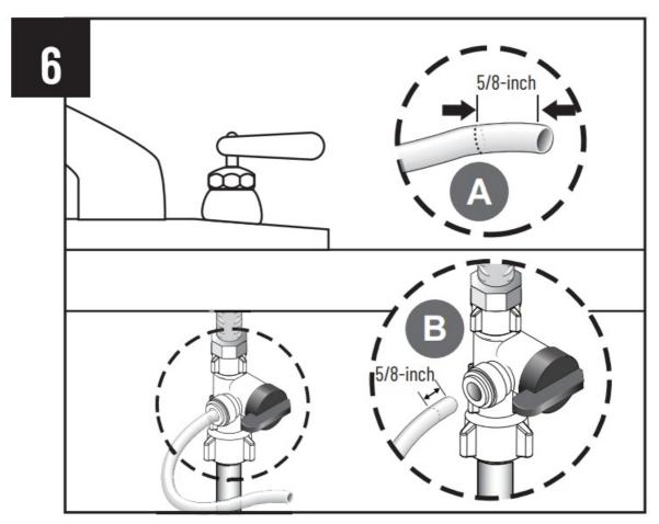
A. Locate remaining length of 1/4-inch plastic tubing. Place a mark on the tubing 5/8-inch from the end. Moisten the end of the tubing with water and insert with a twisting motion push into quick connect fitting on the left side of system. Depending on the installation, the system may need to be removed from the mounting surface to access the left side of the system.
