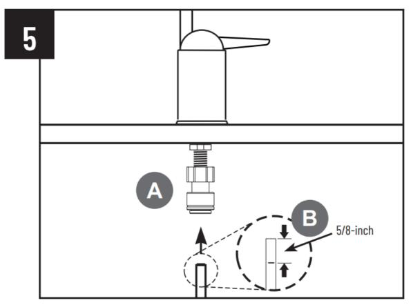
A. Thread flow control onto threaded stem of faucet. (Do not use Plumber tape or sealant.) Tighten flow control hand tight. Finish tightening with a wrench an additional 1/2 turn, do not overtighten.
