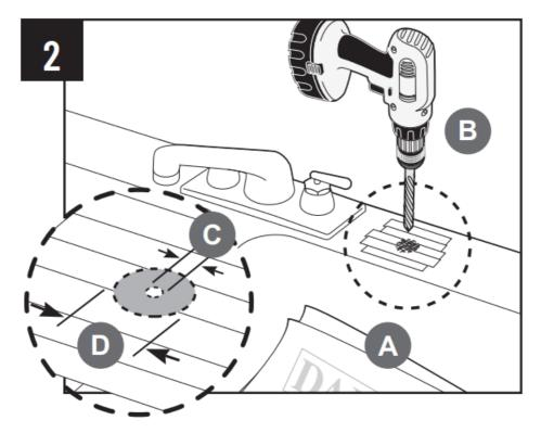
**NOTE:** The drinking water faucet should be positioned with function, convenience, and appearance in mind. An adequate flat area is required to allow faucet base to rest securely. The faucet fits through a 3/4-inch hole. Most sinks have pre-drilled 1 3/8-inch or 1 1/2-inch diameter holes that may be used for faucet installation. If these pre-drilled holes cannot be used or are in an inconvenient location, it will be necessary to drill a 3/4-inch hole in the sink to accommodate the faucet.
