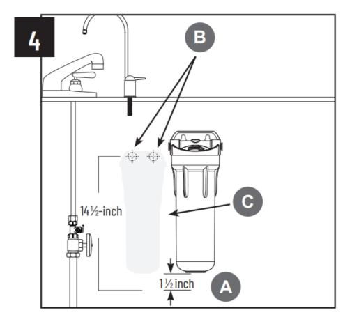
A. Select location under sink or in basement where filter is to be mounted.
