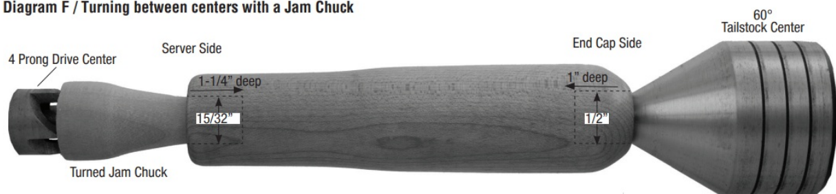
Diagram F / Turning between centers with a Jam Chuck
