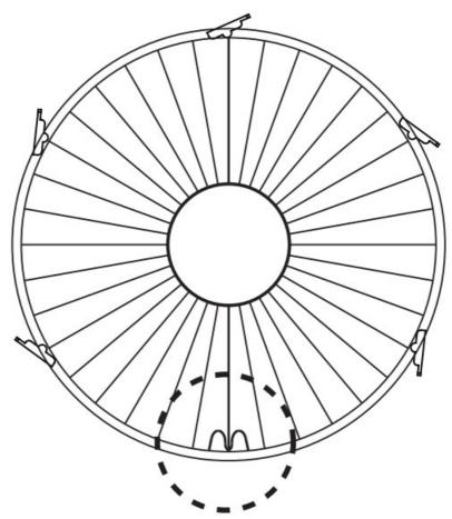
2. Press down all the Buckles to fasten the Front Guard with the Rear Guard. At the Screw Holes, tighten the separated screw and nut.
