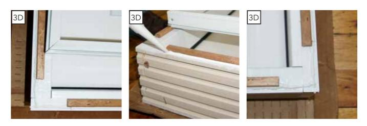
E. Position the assembled clad frame over the molded nose.
