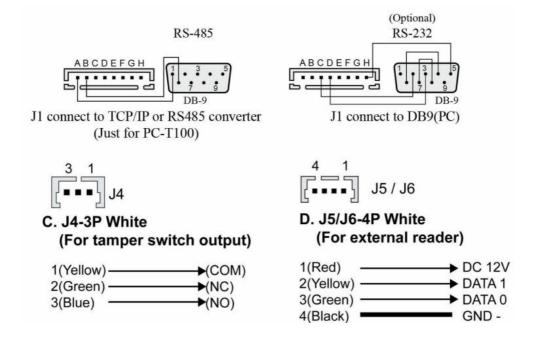
Need to set F4 = 9816, when connect with the external reader that Model No. is included —PW26
