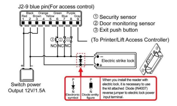
Wiring connection with external relay and power supply for heavy load locks
