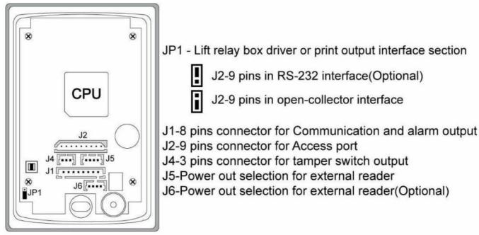
Wiring Connectors and PIN assignment
