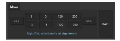
Click each button. Each button represents how many steps the motor is going to move forward (+ steps) or backward (- steps). Notice that the "Position" indicator will change its value and will confirm your command
