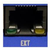
IMPORTANT NOTICE: DO NOT CONNECT ANY MOTOR OUTPUT OF AN EXTERNAL CONTROLLER SUCH AS THE ULTIMATE POWER BOX OR DUAL-MOTOR FOCUS INTO THE RJ45 PORT. THIS MIGHT CAUSE SEVERE DAMAGE TO THE DEVICE
