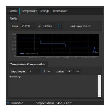
You can easily check what was the last focus temperature so you will estimate if it is time to refocus. Usually, a temperature difference of 2 degrees demands a telescope re-focus. (Lots of factors rule this decision such as type of glass, carbon or aluminum tube, etc.)
