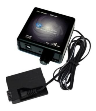
DSLR Buddy is a compact device designed to provide constant power to your DSLR camera. It can accept DC voltages between 3V and 14V and always regulate the DSLR Output to 8V DC. Power can be inserted into the micro-USB socket or to 2.1mm socket.
