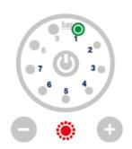
The LED (from 1 to 7) lights up. Corresponding to the number of the alarm.
