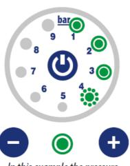
In this example the pressure indicated is 3.5 bar.
