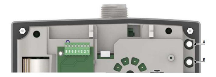
• Use cable entry/exit points A and B to pass the signal cables to connect to the expansion card.
