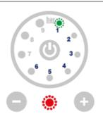
The LED that flashes (from 1 to 6) corresponding to the alarm number.
