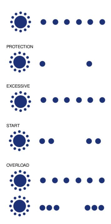
PRESFLO MULTI features 2 LED indicators to show the system's operating status and alerting to any issues through blinking patterns. A guide on the electrical panel helps to identify specific problems indicated by the LEDs.
