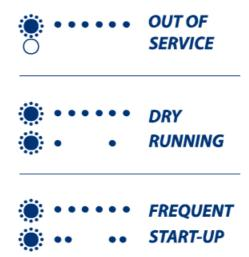
The EASYPRESS features 2 LED indicators to show the system's operating status and alert to any issues through blinking patterns. A guide on the user interface helps to identify specific problems indicated by the LEDs.
