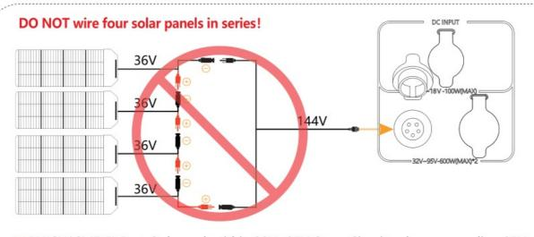
X PV(GX16MF-5) Port Only work within 32V~95V Open Circuit voltage, exceeding 95V will damage the machine.
