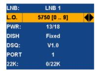
3. Use LEFT/RIGHT to select dish type: Fixed/Moved/UnicableLNB A/Unicable-LNB B.
