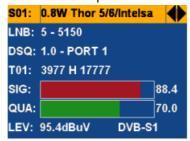
1. Press OK to display signal information, such as level, Carrier/Noise ration and the Bit/Error rate.
