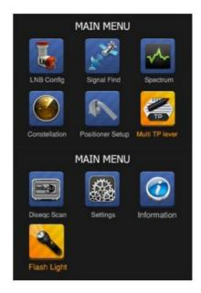
Navigate with the arrow keys (right, left, up and down) to select the desired function and confirm the selection with the OK button. In the main menu you will find the various search functions for LNBconfiguration, Signal Find, Spectrum analyzer, Constellation, Positioner Setup, Multilevel, DISEqC-Scan, Settings, Information (Battery display, Factory settings, short manual, serial-number, firmware-version), Flashlight.
