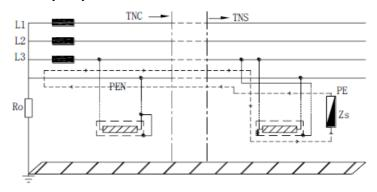
If there is an RCD or fuse in the circuit, it should test loop impedance. According to IEC 60364, every loop should meet the formula:
