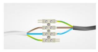
Depending on the flush-mounted box, some- times it is necessary to extend the 230 V side of the power supply. Use the Controlpro 230 V connection set, also available in the shop.
