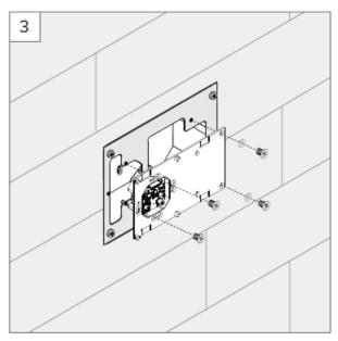
• Insert the panel into the mounting plate and, if necessary, fasten the grub screws to prevent theft.
