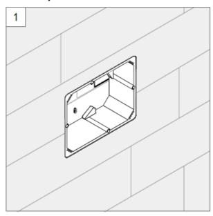
• Fasten the Merten Touch Panel 7 adapter plate to the flush-mounted box using the associated Merten mounting screws.
