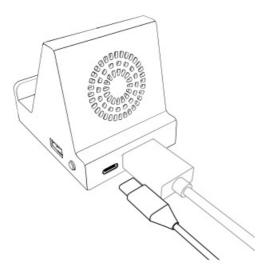
**Note** If you want to support remote touch control of the PeakDo handhelds, the USB cable needs to be connected to a Windows computer or Android tablet.
