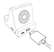
2. Connect the USB cable to the USB Type-C port on the back of the dock, and connect the other end to the power supply port (such as charger, computer, game console, tablet, etc.).
