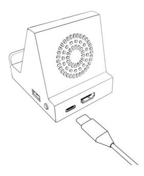
**Note** If you want to support remote touch control, the USB cable needs to be connected to a Windows computer or Android tablet.
