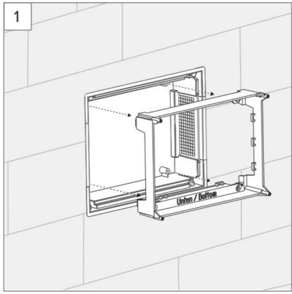
2. Attach the adapters directly to the Gira Control 9 Flush-mounted box. Use Use the Gira mounting screws for fastening. Plug the adapters directly into the Gira Control 9 flush-mounted box. Use the Gira screws for
