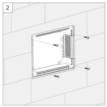
3. Attach the GiraControl 9 adapter plate to the flush-mounted box with the included mounting screws. Fasting the Gira Control 9 adapter plate to the flush-mounted box using the supplied mounting screws.
