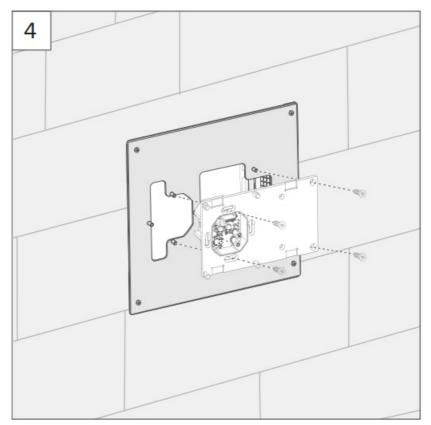
5. Attach the panel to the mounting plate and If necessary, fasten the grub screws to protect against theft. Insert the panel into the mounting plate and fasten the grub screws to prevent theft.
