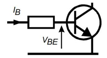
The forward base-emitter voltage drop can aid in the identification of silicon or germanium devices. Germanium devices can have base-emitter voltages as low as 0.2V, Silicon ypes exhibit readings of about 0.7V and Darlington transistors can exhibit readings of about 1.2V because of the multiple baseemitter junctions being measured.
