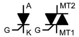
Sensitive low power thyristors (Silicon Controlled Rectifiers – SCRs) and triacs that require gate currents and holding currents of less than 5mA can be identified and analysed ith the DCA55.
