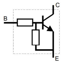
Digital transistors aren't really digital, they can act in both a linear or fully on/off mode. They're called "digital transistors" because they can be driven directly by digital utputs without the need for base current limiting resistors.
