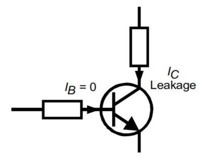
Older Germanium types however can suffer from significant collector leakage current, particular at high temperatures (leakage current can be very temperature dependant).
