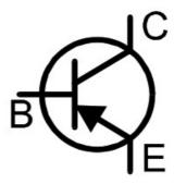
Bipolar Junction Transistors are simply "conventional" transistors, although variants of these do exist such as Darlingtons, diode protected (free-wheeling diode), resistor shunted types and combinations of these types. All of these variations are automatically identified by the DCA55.
