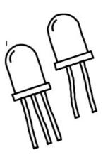
Bicolour LEDs are automatically identified. If your LED has 3 leads then ensure they are all connected, in any order.
