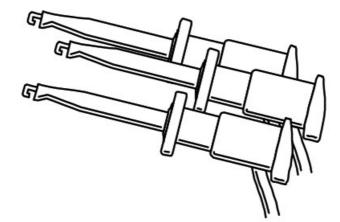
The DCA55 is designed to analyse discrete, unconnected, unpowered components. This ensures that external connections don't influence the measured parameters. The three test probes can be connected to the component any way round. If the component has only two terminals, then any pair of the three test probes can be used.
