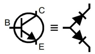
Faulty transistors that exhibit very low gain may cause the DCA55 to only identify one or more diode junctions within the device. This is because NPN transistors consist of structure of junctions that behave like a common anode diode network. PNP transistors can appear to be common cathode diode networks. The common junction epresents the base terminal. This is normal for situations where the current gain is so low that it is immeasurable at the test currents used by the DCA55.
