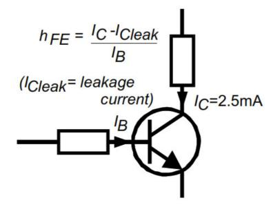
DC current gain is simply the ratio of the collector current (less leakage) to the base current for a particular operating condition. The DCA55 measures hFE at a collector current of 2.50mA and a collector-emitter voltage of between 2V and 3V.
