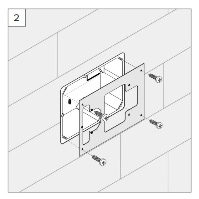
3. Plug the 24 V cable wires coming from the power supply unit into the screw terminals (GND, 24 V) of the Controlmicro mounting plate. Connect the KNX and the network cable. Attach the Controlmicro mounting plate to the adapter using the screws provided.
