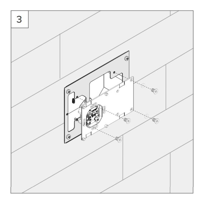
4. Insert the panel into the mounting plate and, if necessary, fasten the grub screws to prevent theft.
