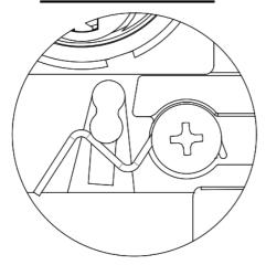
• 09 Function: Extension spring to go around boss on locking mechanism
