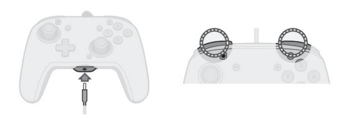
A. Plug the 3.5mm jack of your headset or headphones directly into the 3.5mm port on the controller.
