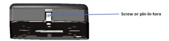
Install the #4-40 screw or pin-in-torx at the bottom of the reader
