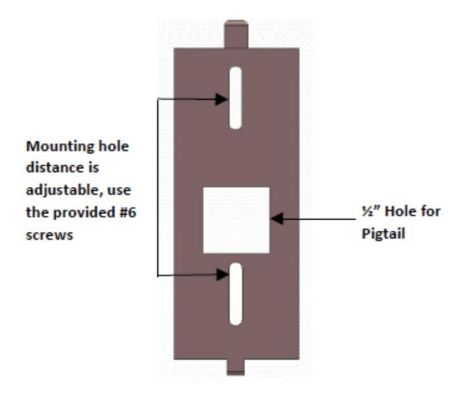
Drill two mounting holes at a minimum of 1.7" apart. Drill a  $\frac{1}{2}$ " hole in the center for the pigtail wire to pass through. Use the wall plate as a guide for drilling.
