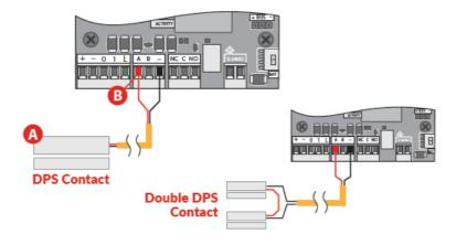
• A DPS (Door Position Switch) - The DPS is mounted on the door frame in the desired location with a 22/2 wire
