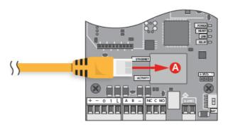
A Ethernet – All Red controllers come with a built in RJ45 connection for network connectivity. Once connected the Red 1 controller is
