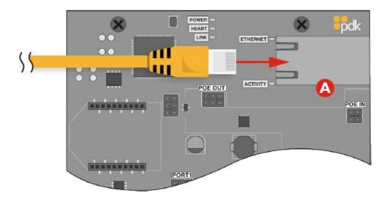
• **A: Ethernet** – Red controllers accept RJ45 connections. The Red 2 controller will be Self-Discoverable from Pdk io software. You have the option to assign a Static IP address but is not required.
