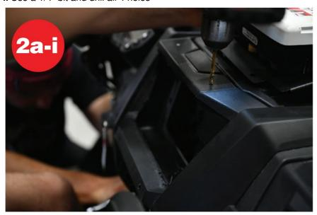
**b.** Mark and cut dash so the back of your **GPS** can recess into the hole.
