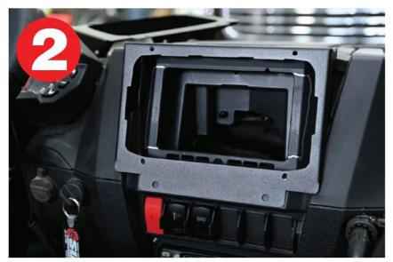
**a.** Mark the 4 mounting holes with a silver sharpie. There are two on top and two on the bottom.
